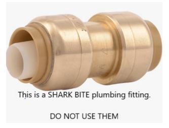
end of that fitting is an O ring type of seal. The only thing holding the water back from leaking is that seal. As with all seals of this type, they eventually fail. Ours failed in 2 years. That was leak # 1.
